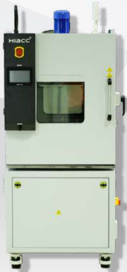
Climatic Test Chamber
