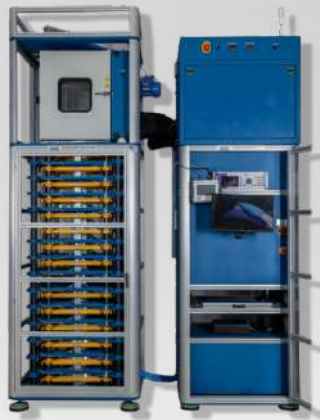
Integrated Temperature Chamber with Force Calibration System
