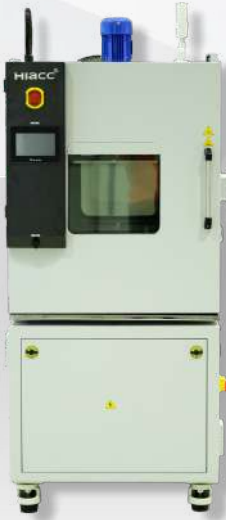
Climatic Test Chamber
