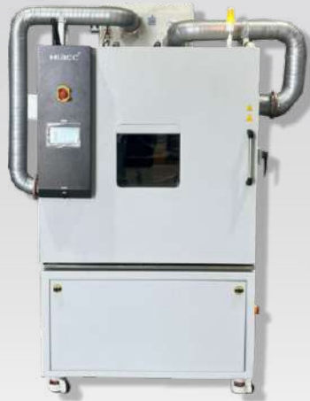
Environmental Chamber with Ultra-Low Humidity Control
