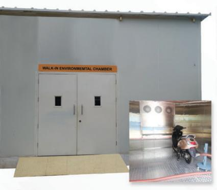
Walk-In/Drive-In test chambers simulates multiple environmental exposures on a whole vehicle or it's assemblies. Walk-In Chambers are designed and assembled using pre-farbricated modular panels or through welded floor construction. Appropriate construction type is selected based on the specimen type and test profile.
